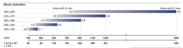
The air flow rates and the pressure drop rates are certified according to the UNI 8728 and prEN 12238 standards, by an independent and certified body, in compliance with the legislation in force on energy saving standards.
