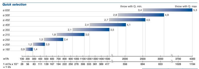
The air flow rates and the pressure drop rates are certified according to the UNI 8728 and prEN 12238 standards, by an independent and certified body, in compliance with the legislation in force on energy saving standards.
