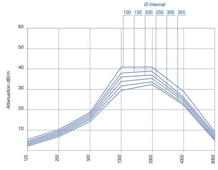
Frequency per octave band (Hz) - Insulation 25 mm
