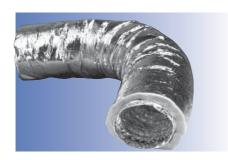
Internal duct like AL 1, micro-perforated, thermally and acoustically insulated by a 25 mm thick glass fiber layer. Externally protected by glass fiber reinforced aluminium laminated foil.
