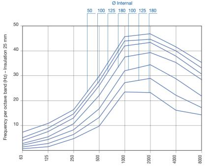
Attenuation dB/m (length of duct 2 m. max)
