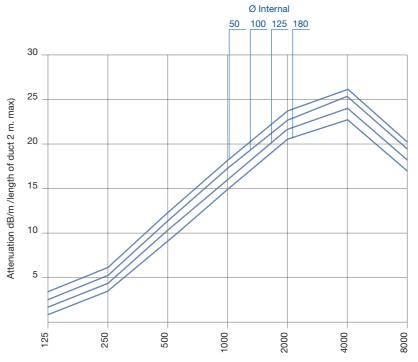
Frequency per octave band (Hz) - Insulation 25 mm
